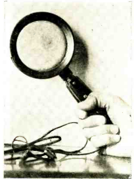
Fig. A One model of the "Radiophon," showing the reproducing surface above the handle.
