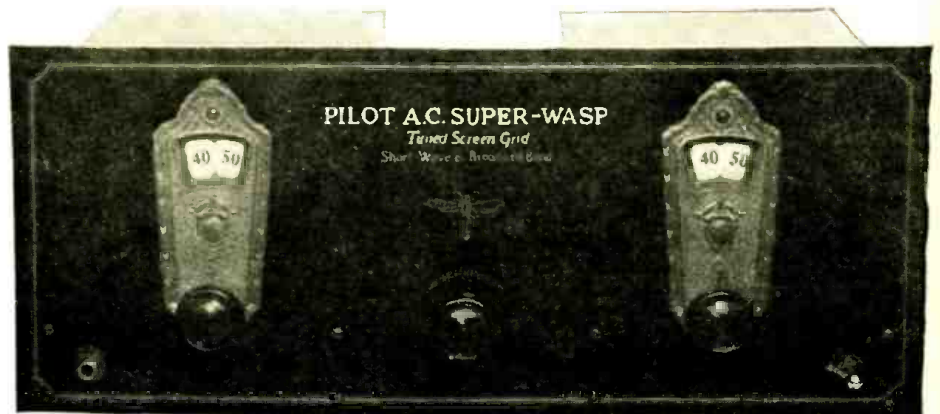
The attractive appearance of the "A.C. Super-Wasp" in its metal-paneled cabinet, is shown above. The jack permits the use of phones, which are desirable for tuning, as well as a loud speaker.
